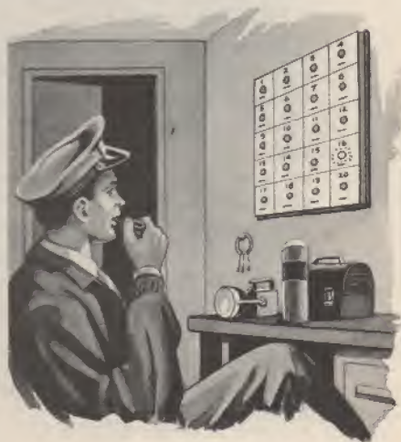
Trained dogs walk up and down the aisles of a department store at night (left). A guard watches the board in a separate room (right) where light bulbs light up as the dogs break the invisible light beams crossing the aisles.
